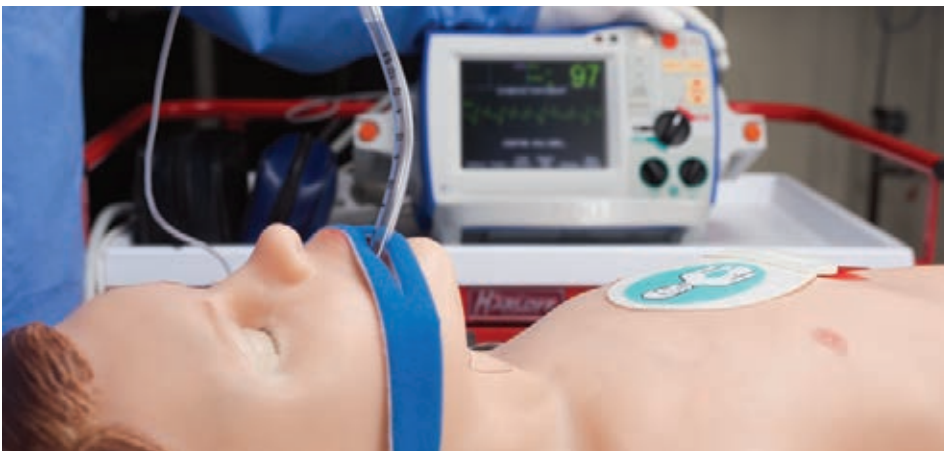
Defibrillation, cardioversion, and pacing using real devices and live energy
